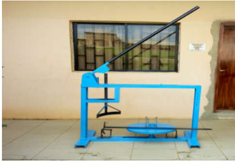
Figure 2: Fabricated Tyre Bead Breaking, Removal and Insertion Device
