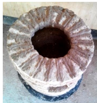
Plate 13: Completed modified furnace
