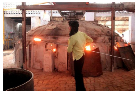
Plate 2: A Pot Furnace in Firozabad Source: [8 Shafi]
