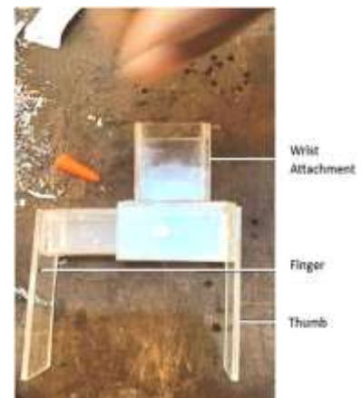
Figure 15. The Fabricated Gripper (without the motor and the rubber padding)
