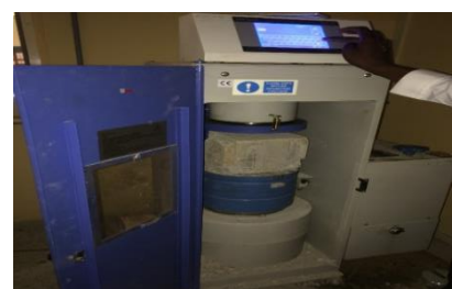
Figure 8: Concrete cube test
