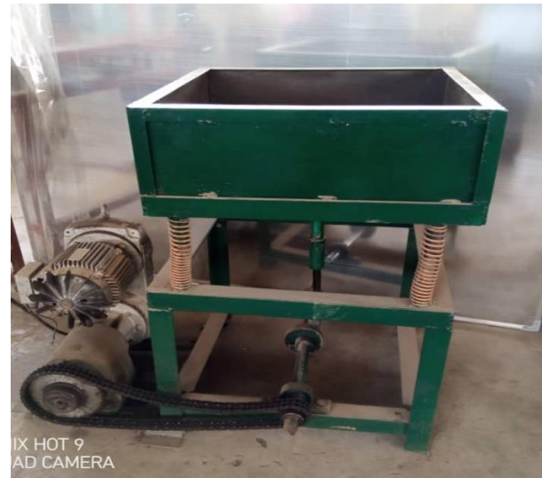
Plate 1: View of the established variable amplitude and frequency of the vibrating container.
