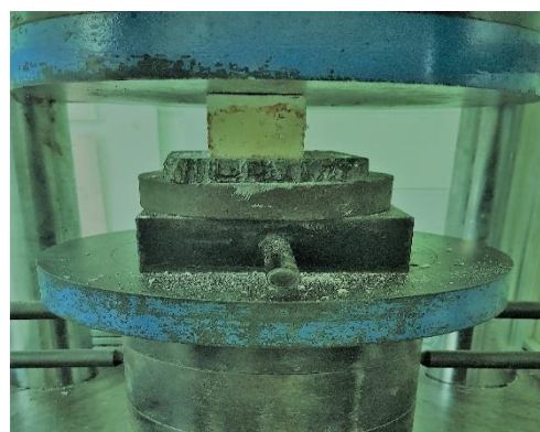
Figure 3: Compressive machine according to ASTM C473-12.
