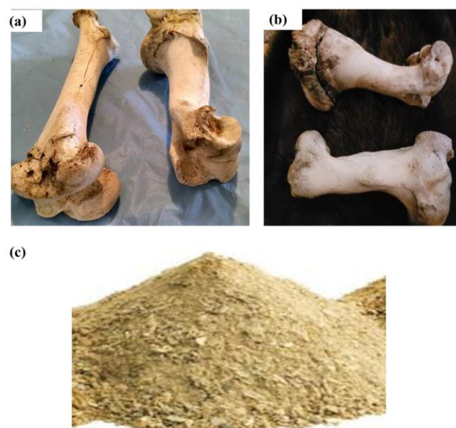
Figure 3: : Cowbone samples processes: (a) sourced; (b) cleaned and washed; and (c) ground into a powder [21].
