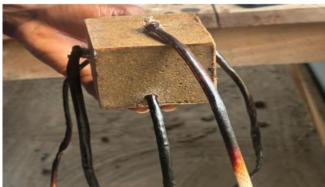
Figure 1: Reinforced Composite Sample with Type-K Thermocouples Inserted.
