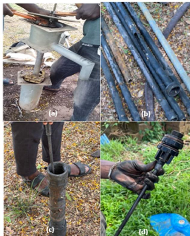
Figure 2: Components of Dismantled Hand Pump (a) Discharge Pipe, (b) Suction Pipes with Sockets, (c) Pump Cylinder, and (d) Connecting Rod with Socket
