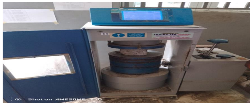
Figure 4: Compressive Strength Machine
