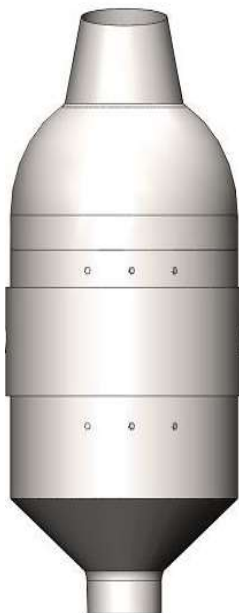
Figure 8: 3D View of the Converter Shell
