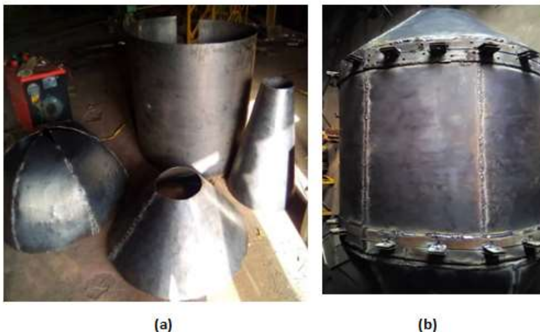
Figure 12: Parts of the Converter Shell (a) before and (b) after Welding, and Fastened Hinge with Bolts and Nuts.
