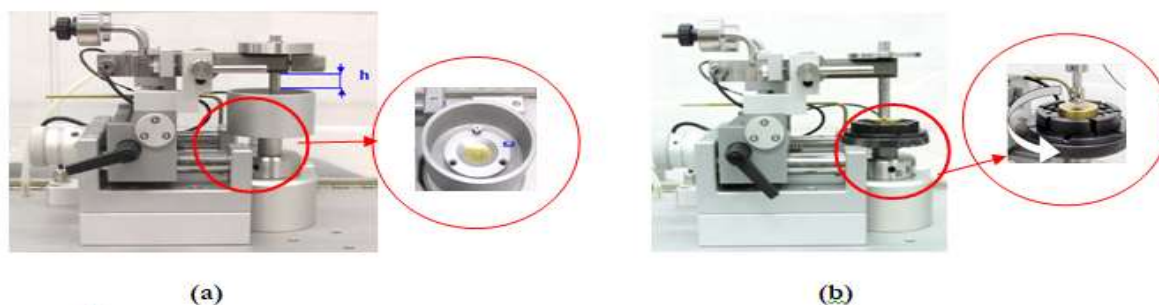
Figure 2: The laboratory set up for (a) wet wear and (b) dry wear test (Anton-Paar G74IB001EN-B User manual)
