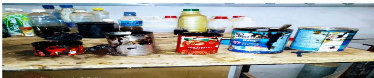
Plate I: The prepared bituminous paint blends in various containers
