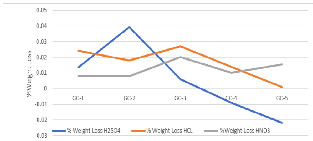
Figure 3: Effect of gradual \text{Al}_2\text{O}_3 addition on the chemical durability of glass-ceramic samples in 1 M \text{HCl} , 1 M \text{H}_2\text{SO}_4 , and 1 M \text{HNO}_3 solutions.
