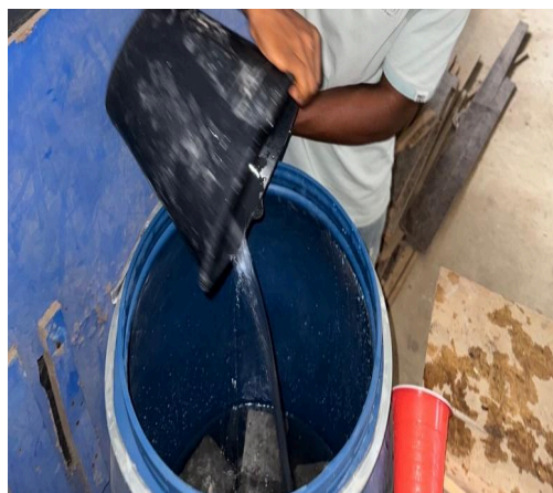
Figure 5: Curing under 2.5% NaCl Solution
