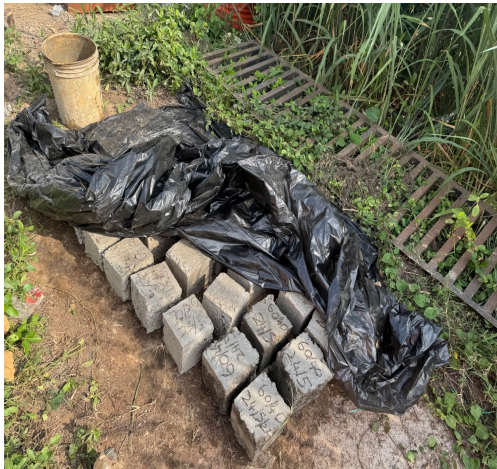
Figure 1: Concrete Cubes Cured under Polyethene Sheets
