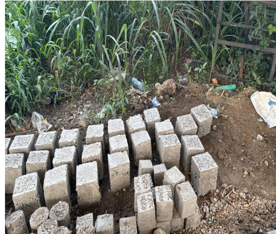
Figure 3: Concrete Cubes under Atmosphere
