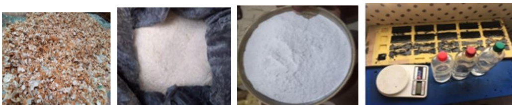
Plate (a) Dry egg shell (b) Milled egg shell (c) Milled glass (d) Scale, epoxy resin, hardener & mixed samples
