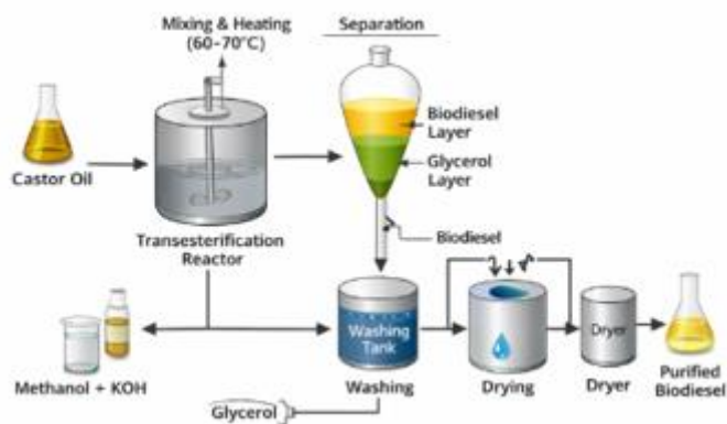
Figure 1: Schematic diagram of biodiesel production process [18]
