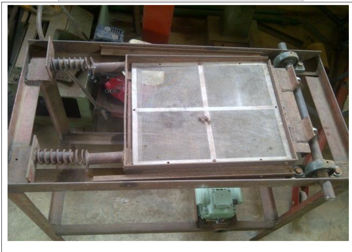
Plate 1: Pictorial view of the fabricated garri sieving machine
