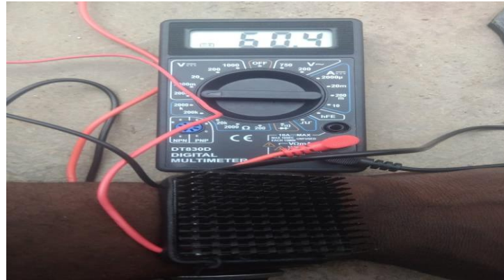
Figure 7: Outdoor test setup with the TEG attached to the wrist
