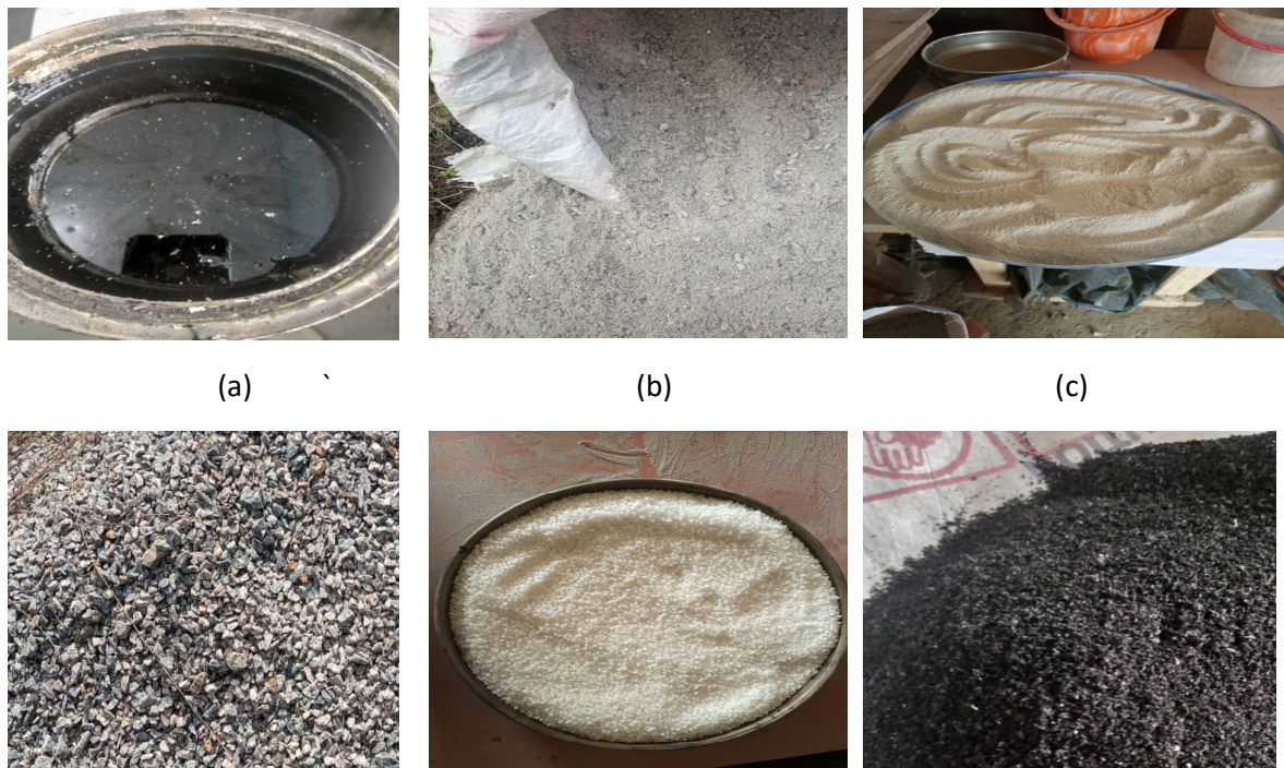
Figure 1: Materials utilized during the research (a) Bitumen sample (b) Fine aggregate sample (c) Conventional mineral filler sample (d) Coarse aggregate sample (e) Sasobit sample (f) Crumb rubber sample
